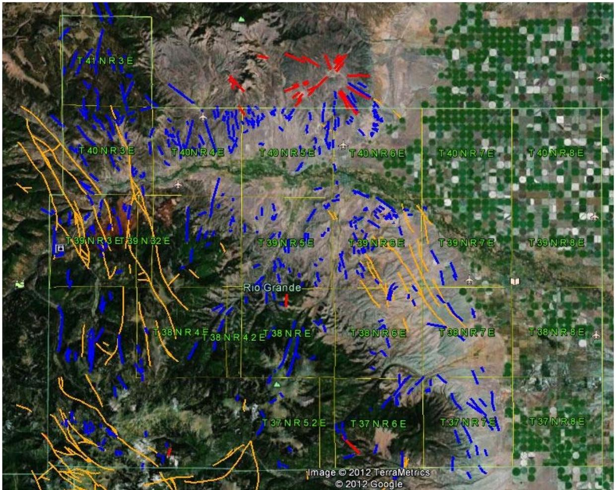
Figure 1. Screen-capture of identified lineaments (blue) and mapped faults (orange) and igneous intrusions (red) in the Rio Grande County hydrogeology study area.
